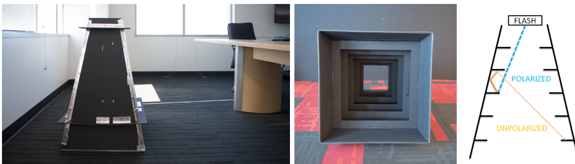
Figure 13: (left) The Perplexicon: a light-tight box made of black foamcore. (center) Baffles reflect and redirect light away from sample. (right) Side-view showing light path.
