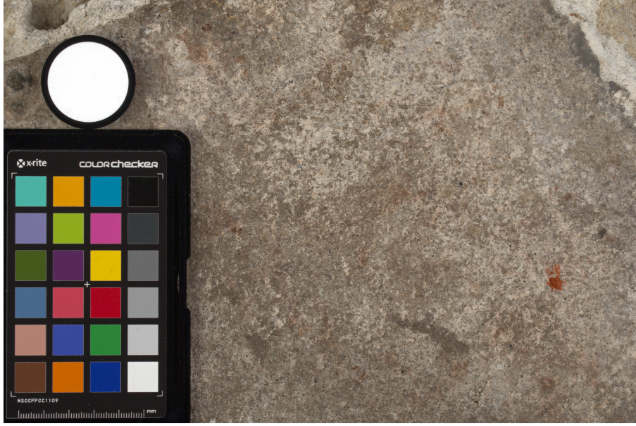
Figure 11: An example of diffuse capture of a concrete material. Notice the perfectly white Spectralon in the top left corner.
