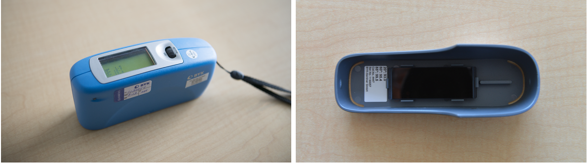
Figure 14: Left: Glossmeter used to measure glossiness of materials. Right: The black glass used to calibrate the glossmeter.
