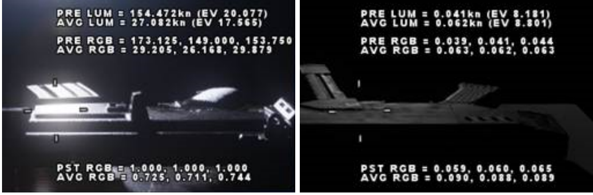
Figure 17: Left: HDR photograph of an airsoft rifle. Highlight measures 17.5EV. Right: Original material used on in-game gun. Highlight measures 8.8EV.
